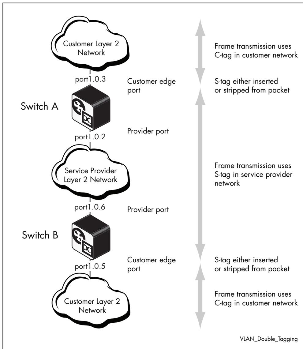
**Configuration procedure for double-tagged VLAN****Step 1: Create and enable the service provider VLAN2**
