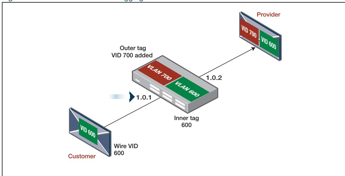
Figure 15: Example configuration for VLAN translation and double-tagging on the same port
